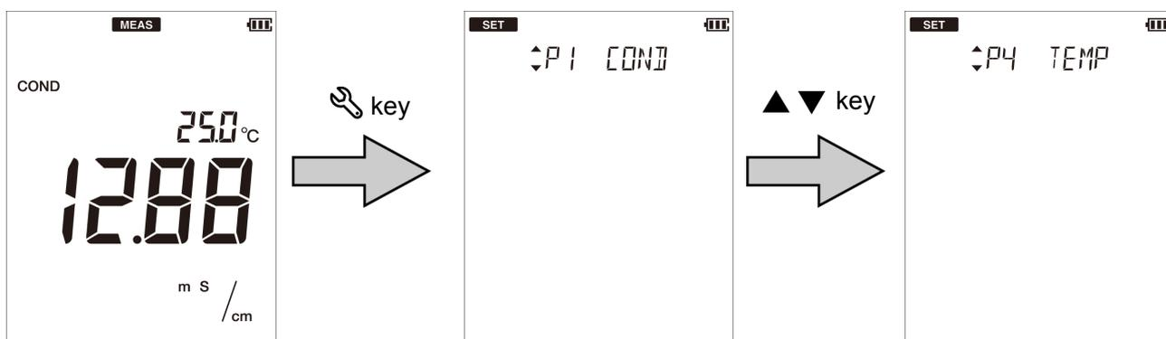
5. Make sure that "ATC" is displayed, and press the
