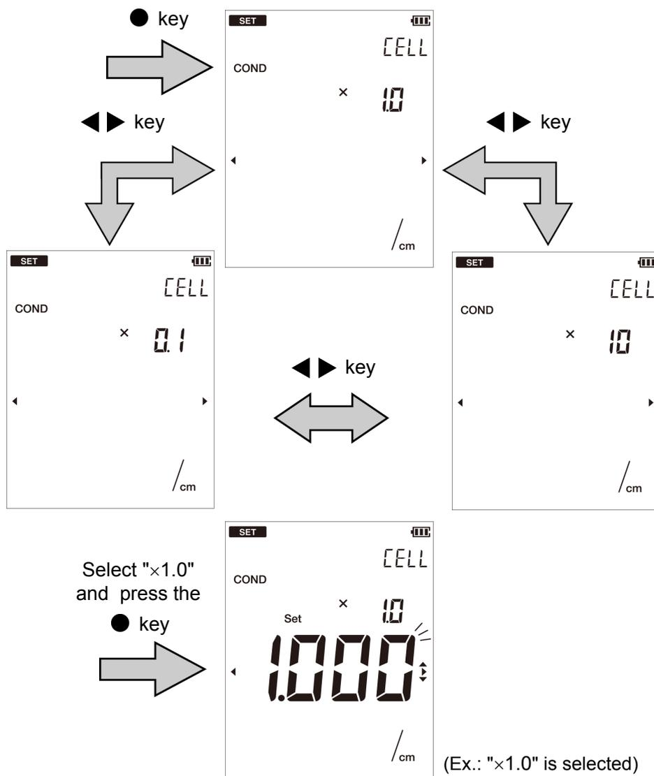
5. Press the ▲▼◀▶ keys to enter the cell constant value of the conductivity cell and then press the ● key to confirm.
