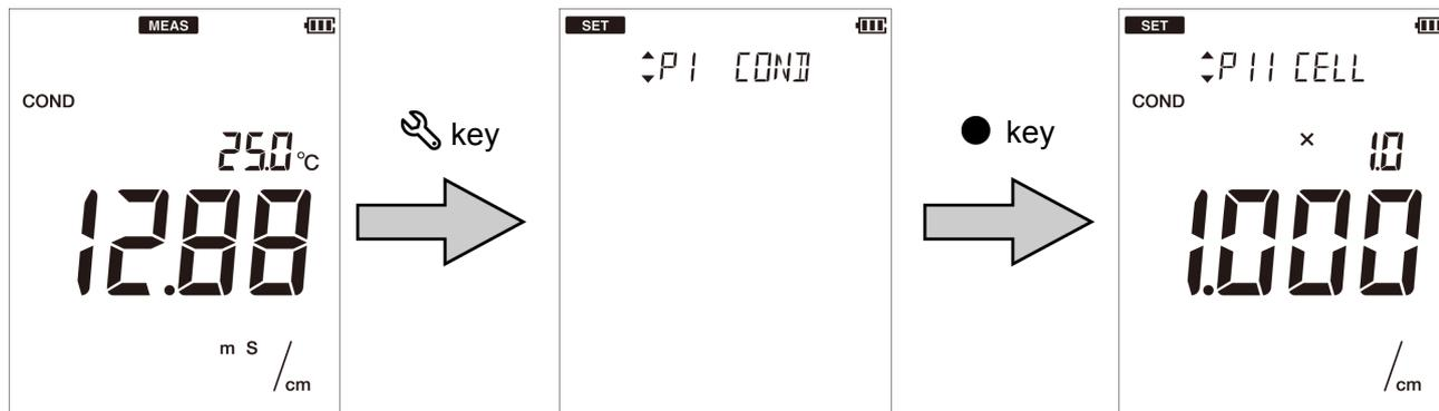
4. Press the ◀▶ keys to select the digit number of the cell constant of the conductivity cell and then press the ● key.
