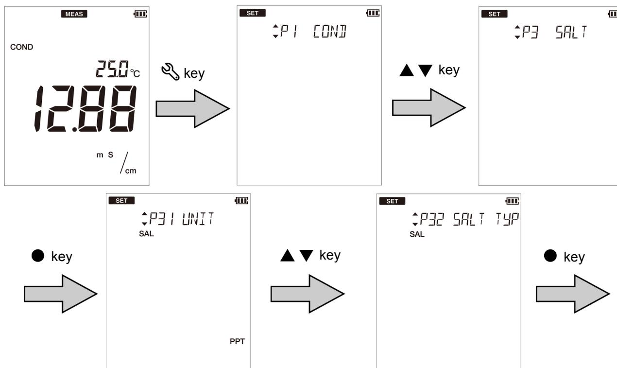
4. Press the ◀▶ keys to select the salinity calculation method and then press the ● key to confirm.
