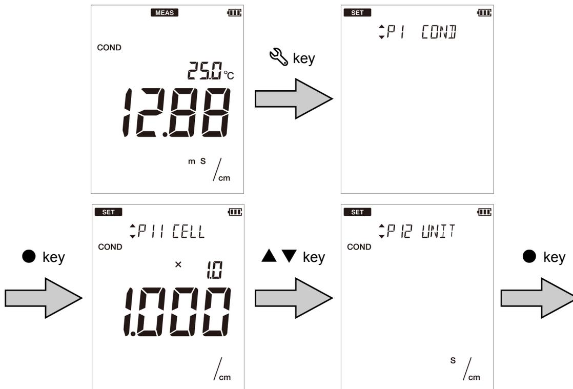
4. Press the ◀▶ key to select the unit and press the ● key to confirm.
