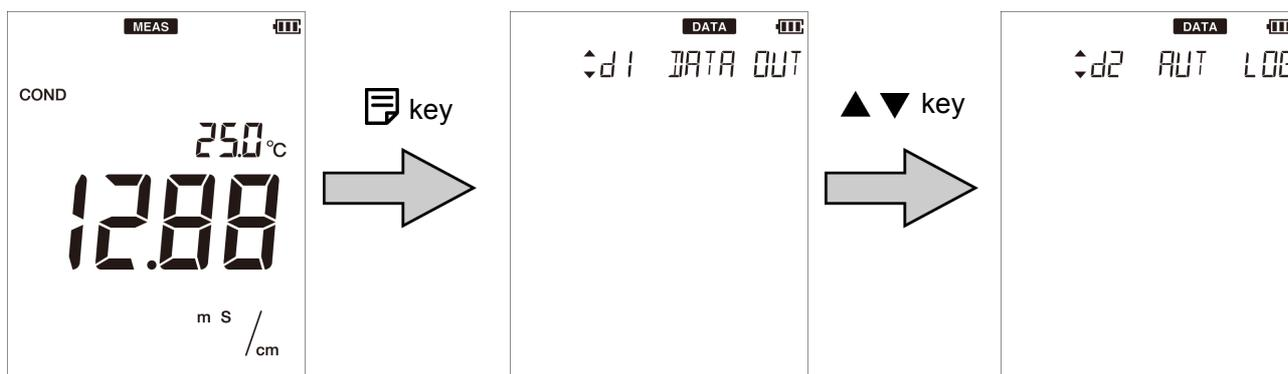
3. Enter the interval of saving in seconds and press the
