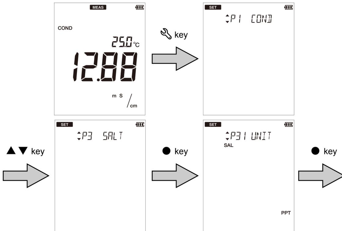
4. Press the ◀▶ keys to select the unit and press the ● key to confirm.
