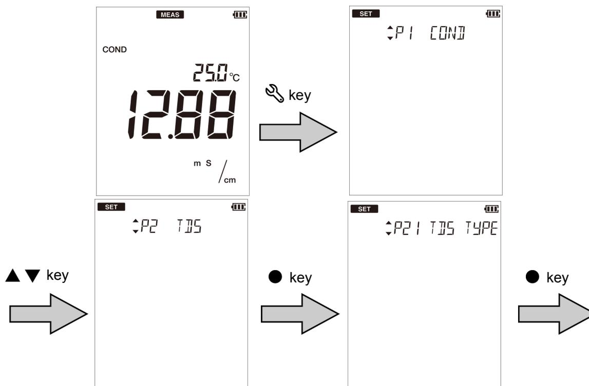
4. Press the ◀▶ keys to select the TDS method and then press the ● key.
